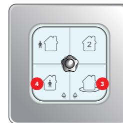
Press buttons 4 and 3 simultaneously. The icons will blink. Place your Smart Key onto the reader.
